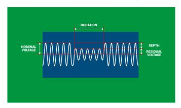
Generally voltage SAG happens when the residual voltage decreases between 10 and 90 percent of nominal voltage for one-half cycle to one minute. Voltage SAG duration is considered within 10ms up to 1min. The great deal of Voltage SAG have a duration lower than 1 second and a residual voltage higher than 40% of the rated value.
